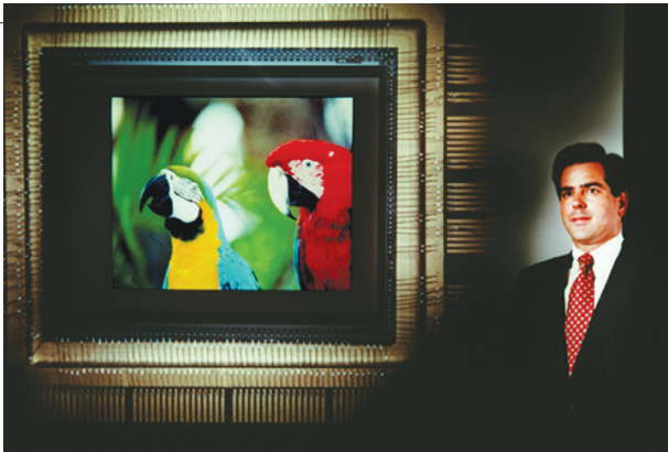
First hidden hinge DMD (1993). The array size is 768 x 576, and the portion projecting an image is 640 x 480. This unique photo captures a historical event, an integrated circuit producing a projected image the size of a man. The field of view of the projection lens was increased to show not only the DMD chip, but also the surrounding package and the bond wires that electrically connected the chip to the package contacts. For size reference, the image diagonal at the DMD chip is 0.53 inches, and the bond wires are one-thousandth of an inch (25 microns) in diameter.
