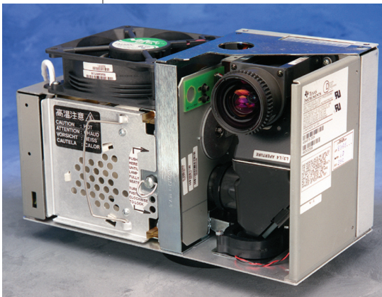
The optical elements of a three-DMD projector (shown without the projection lens). The central structure is a color-splitting and recombining prism assembly. It is surrounded by three DMDs, one dedicated to each primary color (red, green and blue). ] >>
