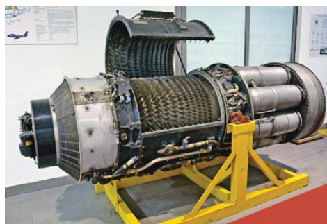
Figure 24 - General Electric J47 turbojet engine, 1948-1956
