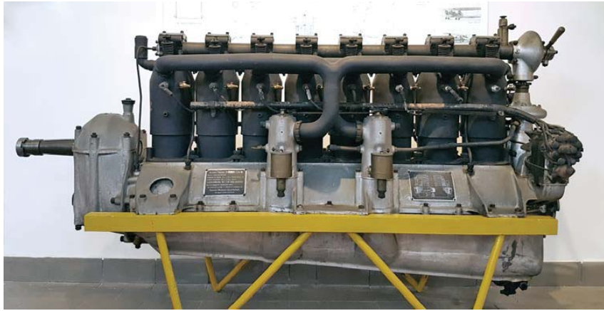
Figure 13 - Daimler Mercedes D.IV aircraft engine, 1916
