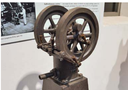
Figure 7 - Stationary Stirling engine, Louis Heinrich Maschinenfabrik, 1905
