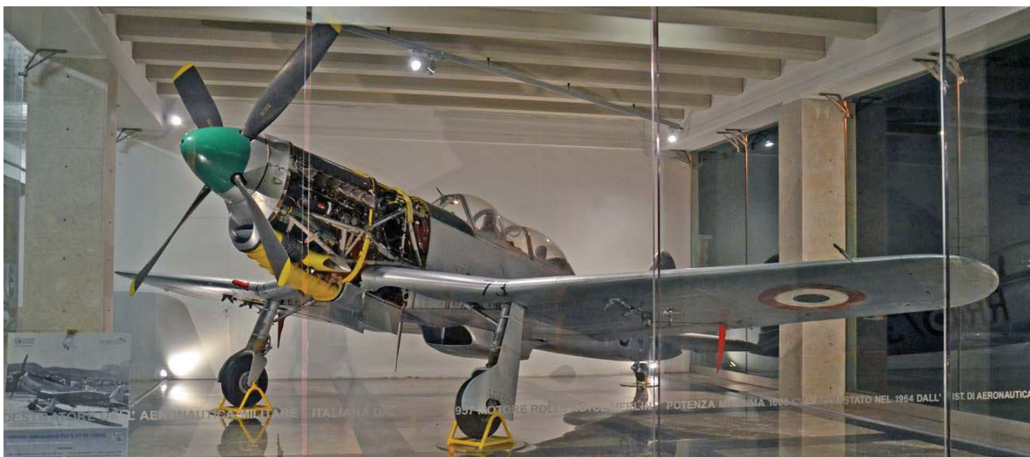
Figure 23 - FIAT G.59 4B trainer aircraft equipped with a Rolls Royce Merlin 500-20 engine, 1950
