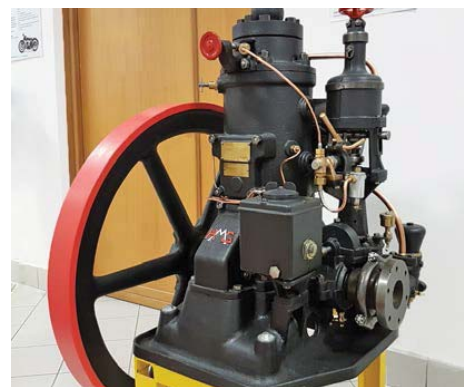
Figure 12 - HMG two-stroke Diesel engine, ca. 1910-1920
