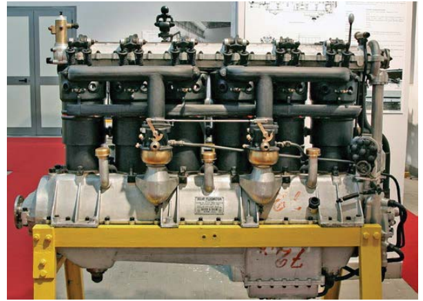
Figure 14 - Basse & Selve BuS.IV aircraft engine, 1917-1918
