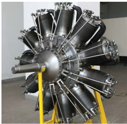
Figure 15 - Siemens Halske Sh.IIIa counter-rotary aircraft engine, 1917-1918
