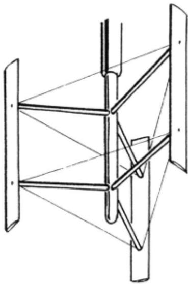
*Darrieus rotor for generating power from a flowing fluid.*
