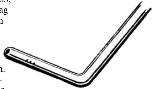
*Pitot tube for measuring local velocity head.*
