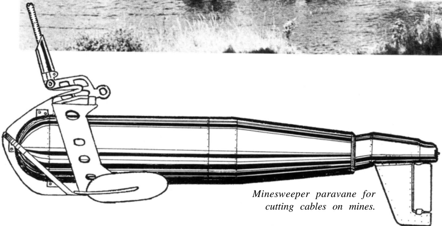
*Minesweeper paravane for cutting cables on mines.*
