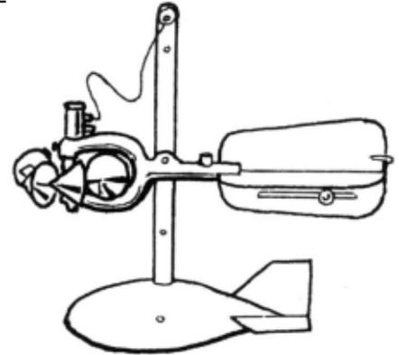
*Typical current meter for measuring flows in rivers and streams.*
