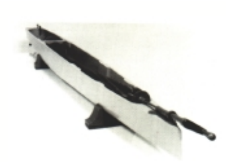
The larger of the two models used by Parsons to determine the hull resistance and power requirements for the Turbinia. Although model testing was still something of a novelty Parsons results were extremely accurate.
