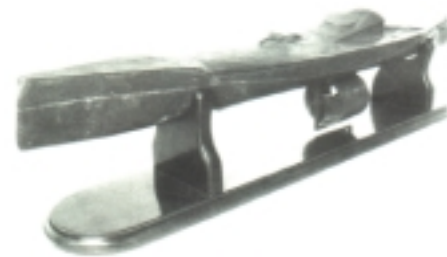
Model launch, reputedly built by Parsons in the early 1880's showing a unique (compressed air-powered) combined underwater turbine/propeller unit. Though not directly related to the Turbinia project it shows his early interest in turbine propulsion for vessels.
