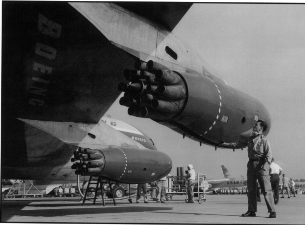
Noise suppressor containing 21 tubes.
