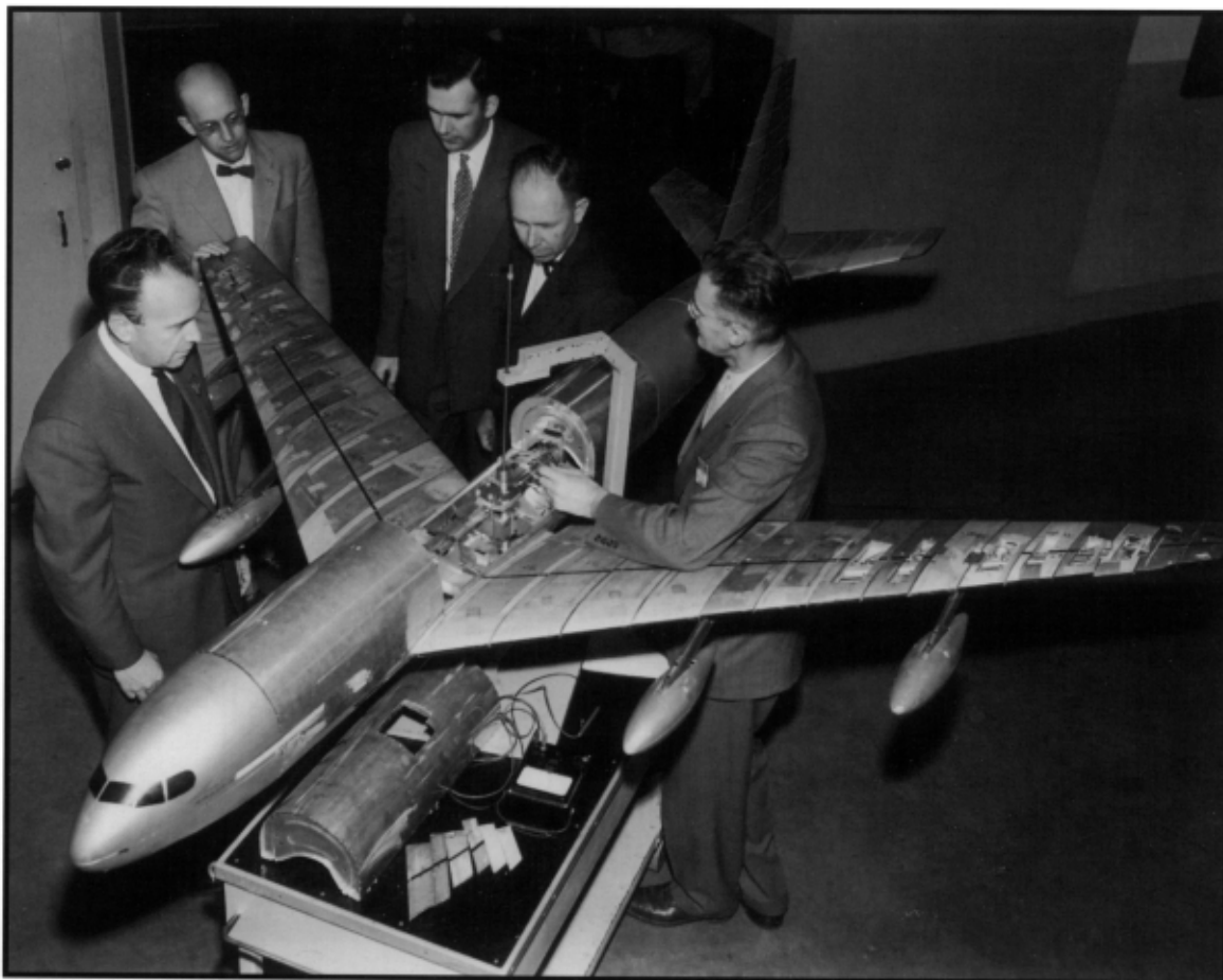
E. C. Wells, G. S. Schairer, J. E. Steiner and M. L. Pennell (left to right) discussing an aeroelastic model with wind tunnel engineer E. Storwick.
