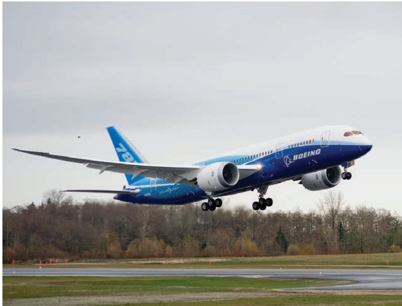
Scalloped engine nacelle trailing edges for noise reduction.
