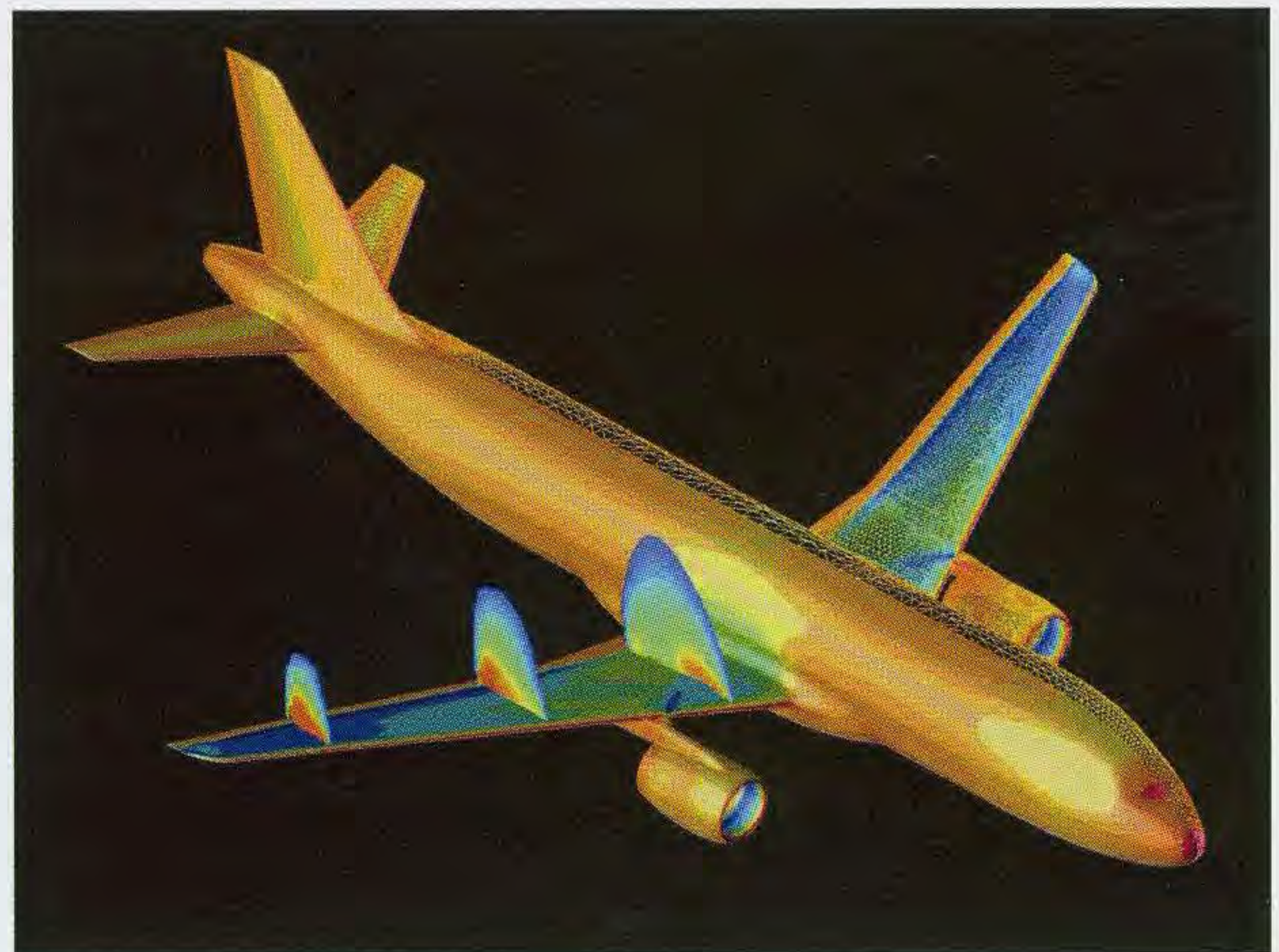
Figure 4 Computed pressure distribution about an Airbus A320. On the right side of the picture the detailed surface triangulation is visible.
