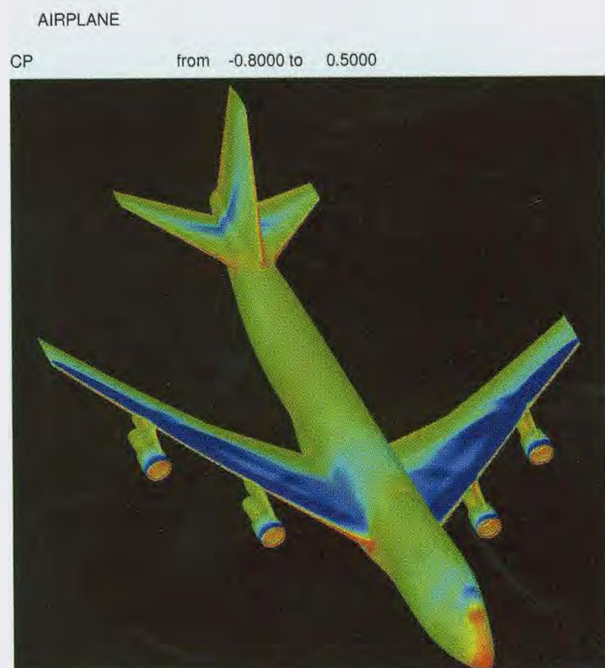
Figure 6. Pressure contours for the Boeing 747-200.
