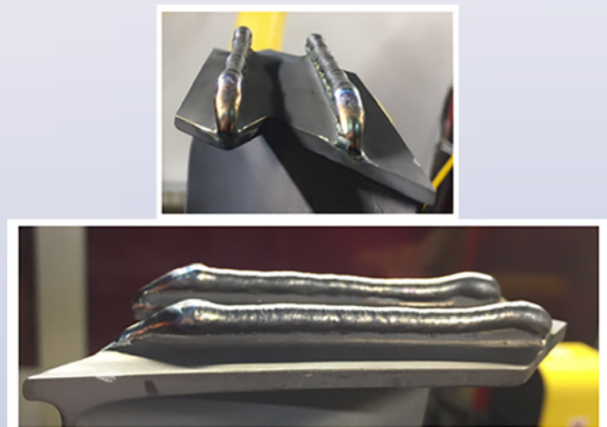
Figure 1. Layer deposition on blade rail tip through CMT technology (front and lateral views)
