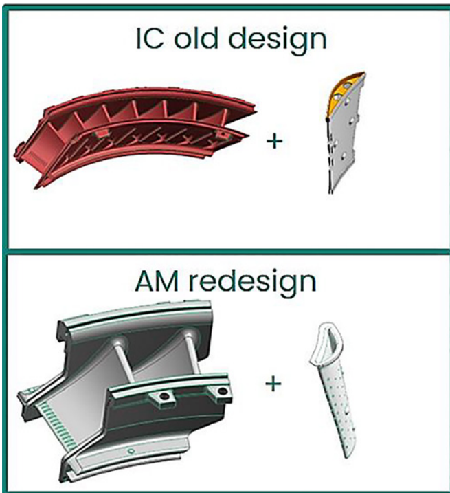
Figure 2. Differences in design for gas turbine nozzle and cooling insert, note that in the AM case the number of airfoils for the sector has changed.
